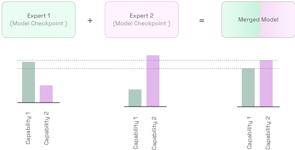
Figure 4: Model merging allows teams to build domain expert models that excel at different capabilities independently. These experts are merged into a single model that retains close-to-expert capability levels across multiple domains or capabilities.
